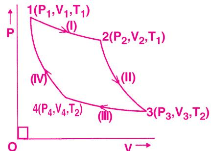
**b) Step II : Adiabatic Expansion(AE) of the gas from  $2(P_2, V_2, T_1)$  to  $3(P_3, V_3, T_2)$ .**
