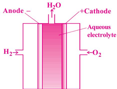
**H<sub>2</sub>-O<sub>2</sub> fuel cell:** This fuel cell consists of porous carbon electrodes suspended in concentrated NaOH solution.
