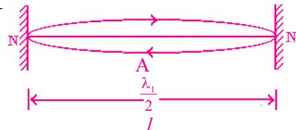
$$\text{We know, velocity of transverse wave is } V = \sqrt{\frac{T}{\mu}}$$
