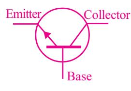
**n-p-n transistor****10. Mention the basic methods of modulation.****A: Basic Methods of Modulation:**
